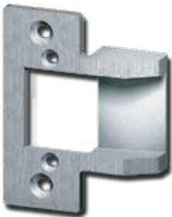
Standard ANSI prep features an extended ramp to accommodate additional face of Timely®/Redi®/Raco®/IDP® frames. Ramp is extended 3/8". For new or replacement installations. Use with cylindrical locksets having up to 5/8" throw, based on 1/8" door gap.
