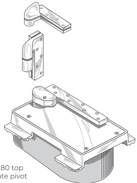
SEC27-180 Closer with FA180 top pivot and FA19 intermediate pivot (recommended)
