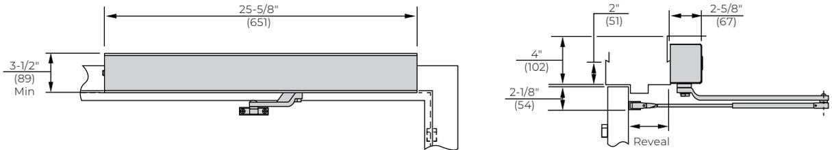
Note: for applications with narrow top rails or limited ceiling clearance, a special drop angle bracket is required. See page 16.
