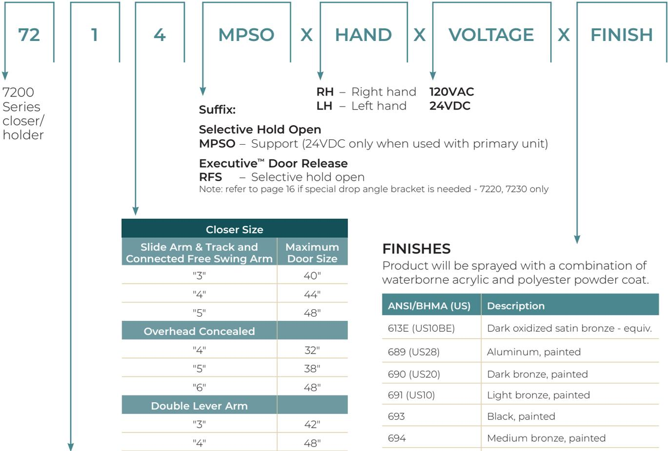
**Specifies side of door unit is mounted on and the type of arm**
