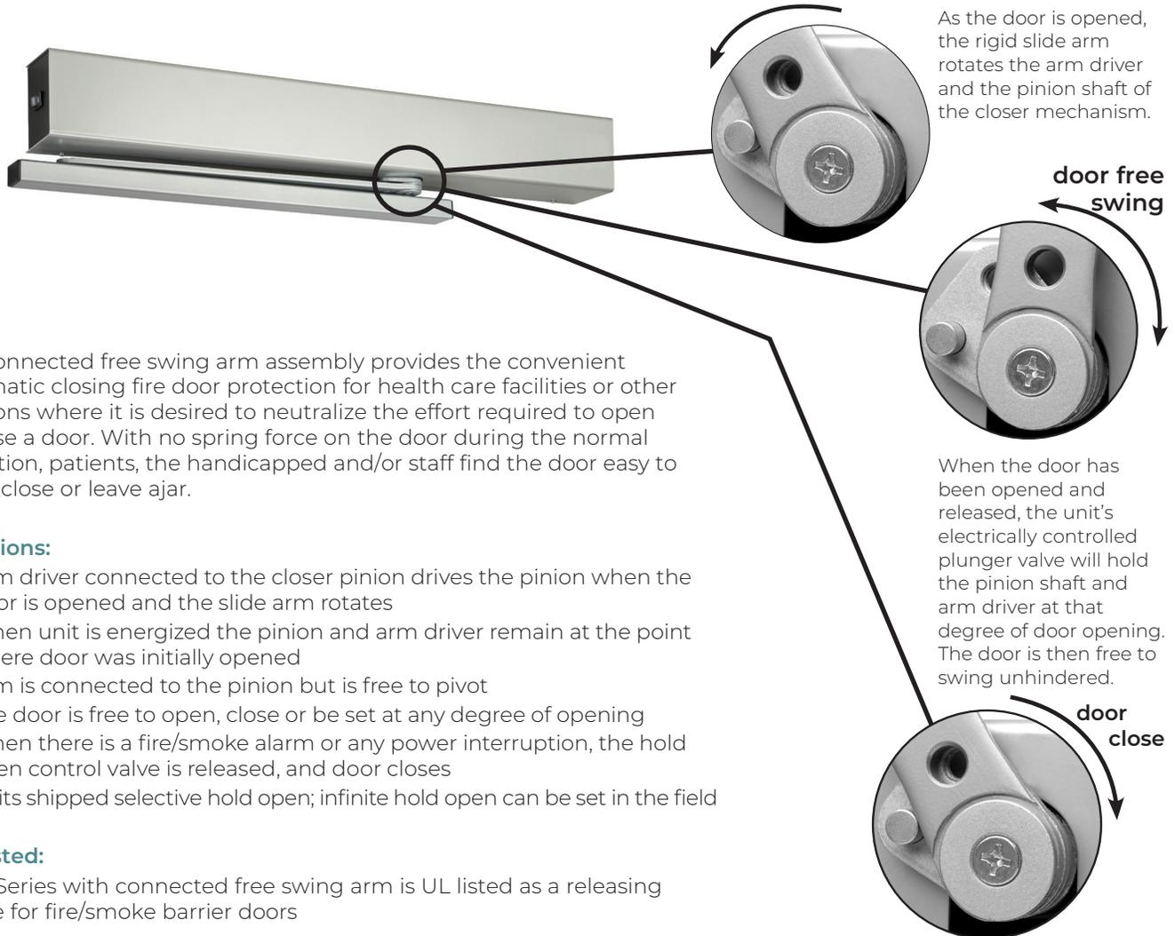
As the door is opened, the rigid slide arm rotates the arm driver and the pinion shaft of the closer mechanism.
