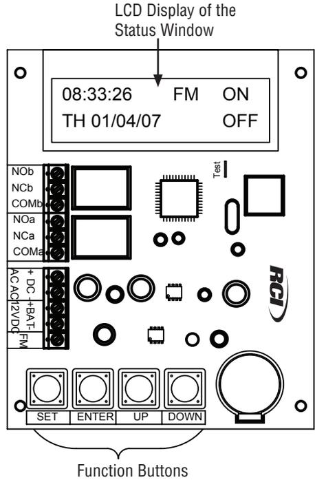
The **Status Window** is the normal screen that will display the time, date, relay state and if the FM function\* has been activated.
