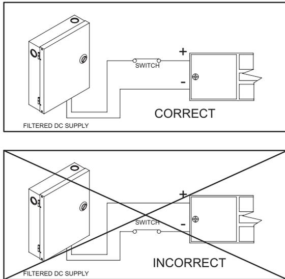
Fig. 2 – Power Connections
