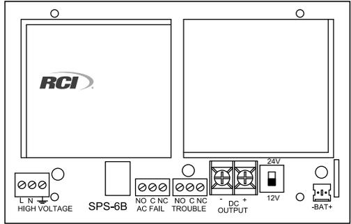
**Fig. 3 -Power Supply Wiring**
