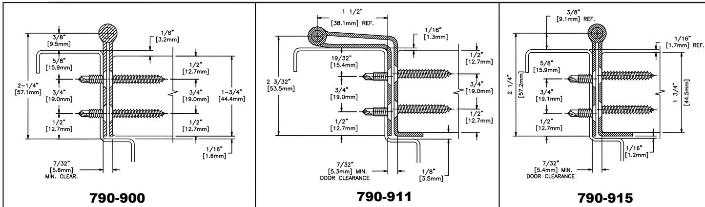
HAGER Models 790-900, 790-911, and 790-915 are Stainless Steel Continuous Edge Mount Hinges for 1-3/4" (44.5mm) thick doors. Clearance required between the hinge edge of the door and the frame rabbet is 7/32" (5.6mm) minimum. Model 790-911 provides 'swing clear' rotation. Models 790-911 and 790-915 feature an integral protective corner guard and are **not** recommended for use on doors that have a beveled edge on the hinge side.
