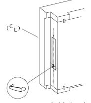
**C-2** Select the strike for the desired handing, according to the depiction on the template. Mark the location of the strike cutout and mounting screws.
