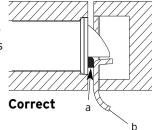
M-2 Mark locations where the gaps are approximately 3/16" (5 mm). Make sure these locations are free from grease and dust. Peel the bumpers (c) (supplied) from their protective backing without touching the adhesive surface and stick them on the marked locations.
