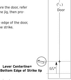
The axis of rotation of the handle is level with the bottom lip of the strike.
