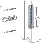
**C-4** Position the strike against the door frame and align it with the mounting screw holes. Then mark the outline of the strike.
