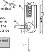
**I-9** Remove the interchangeable/removable cylinder. Then remove the tailpiece (e).
