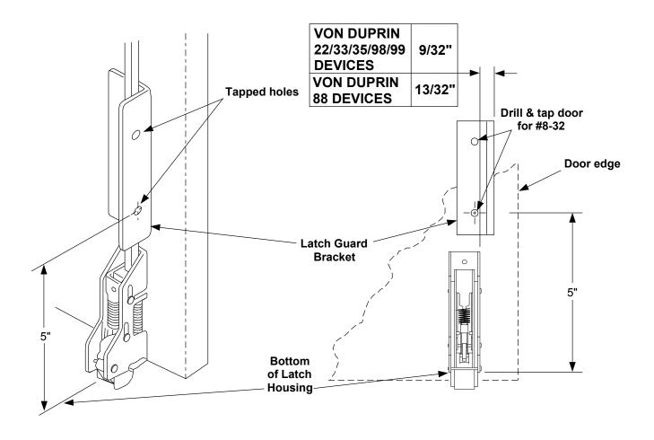
$Step \ \ \ \textbf{3} \ \ \text{Adjust and reinstall vertical rods per manufacturers' instructions.} \ \textbf{Do not install Latch Cover}.$
