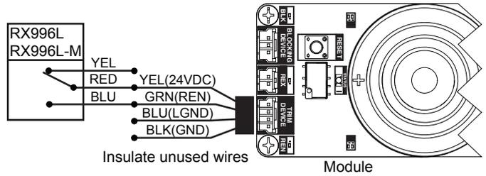
RX trim uses the REN feature to allow entry. It inhibits the DE5300 and unlocks the maglock when the lever is turned.
