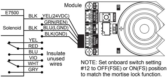
Access control to the DE5300 (not shown) inhibits the DE5300 and unlocks the E7500 mortise lock to allow entry. The E7500 can be either FS (Fail Safe) or FSE (Fail Secure). For access control wiring, see previous wiring diagrams.
