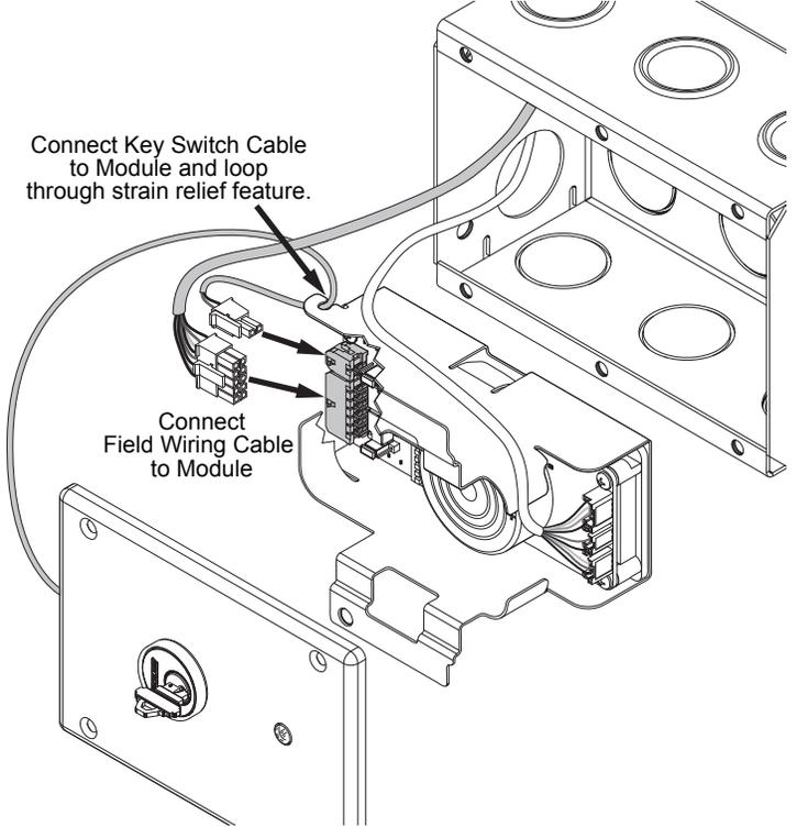
7q Insert mounting bracket with module into control box and screw into place. Screw faceplate into place.
