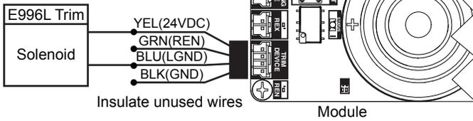
Access control to the DE5300 (not shown) inhibits the DE5300 and unlocks the outside FSE (Fail Secure) trim to allow entry. For access control wiring, see previous wiring diagrams.
