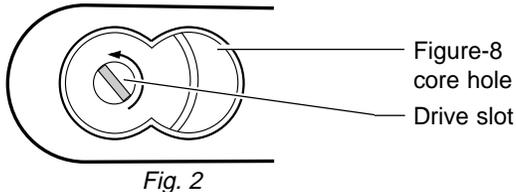
1. Remove both cores and throw members with the control key.
