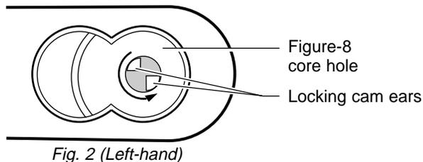
1. Remove the inside core and throw member with the control key.
