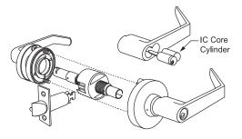
★Standard & HI-SECURITY™ IC Core Models: Interchangeable Core models for 6 or 7 pin cores (not included). Accepts: Marks, Marks HI-SECURITY™, Medeco<sup>®</sup>, KeyMark™, Falcon, Schlage<sup>®</sup> small format & Best<sup>®</sup>. IC Core Tailpieces ARE Included.
