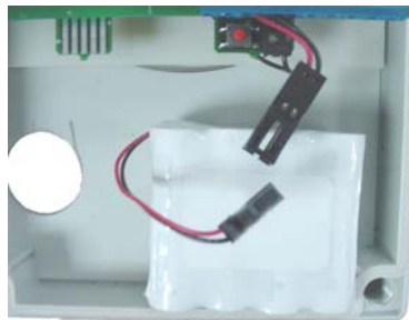
Figure 10-4 – Removing the Used Battery Pack
