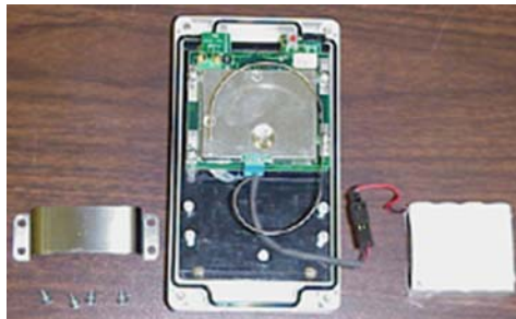
Figure 9-6 - Installing New Battery Pack
