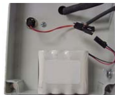
Figure 8-4 – WPR Battery Pack Positioned
