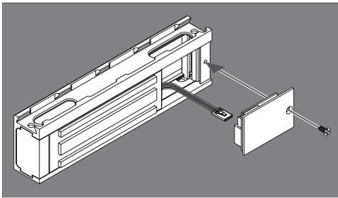
5c Slide magnet onto bracket.
