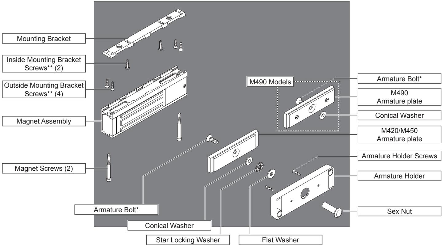
\* M490 Models ONLY: Two armature bolts are included in the package, but only one is used. There will be one left over after proper installation.
