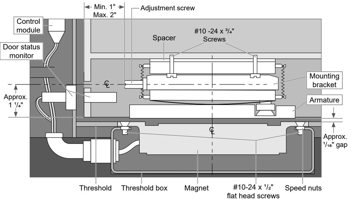
4b Mount magnet into the threshold box.
