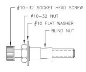
II. Install blind nut assembly into pre-drilled 9/32" hole in door. Hold the socket head screw firmly with the hex wrench to prevent rotations as
