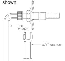
III. Using a 3/8" wrench, rotate the nut clockwise until the nut collapses against the inside of the door skin. Some resistance will be felt. Carefully tighten until nut is secure.
