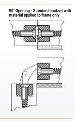
Clearance reduces to approximately 1/64" as door approaches the frame upon opening. Beyond that point, the clearance increases to the maximum clearance when the door reaches its fully open position at 180°. See the hinge template drawing for that dimension. If the template "E" dimension is exceeded, the door will hit jamb and bind. See specifications for SOSS Invisible Hinges on previous pages for dimension "E".
