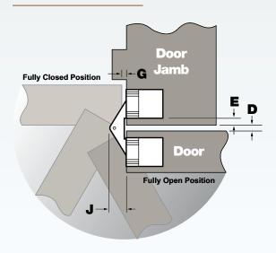
The diagram below left shows the typical path of a SOSS hinged door. The table shows the door clearance when fully opened for each SOSS hinge.
