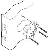
Remove the following from your Hardware Bag: 2 each of the Handle Pivot Screws, 2 each of the Handle Shaft and 2 each of the Cover Screws.
