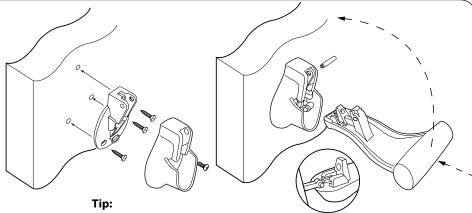
Mark top hole at 12 o'clock. Drill pilot hole and attach with screw to snug, check for level. Mark other screw holes with pencil. Loosen Unirose and rotate 180°. Drill other pilot holes. Return Unirose to original position and install remaining screws.
