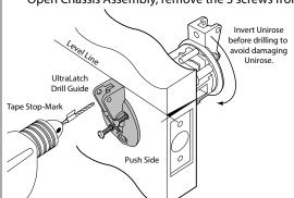
Invert Unirose to avoid drilling into it and place in the 21/8" face hole on door.
