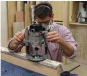
Each router guide template is individually handcrafted for exactness. The template is held on the door and jamb with nails; guide pins locate the deep mortise. The edges of the template assure a perfect outline when used with SOSS RGB100 Template Guide and Lock Nut, or the Porter-Cable Template Guide #42024 (Lock Face Routing) and #42237 (Lock Nut).
