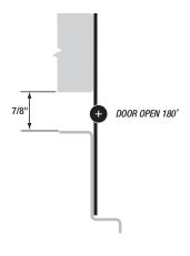
**MATERIAL:** 14 gauge 304 stainless steel with 3/16" diameter 304 stainless pin. Long-life nylon medical bearings.
