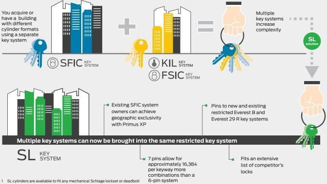
I SL cylinders are available to fit any mechanical Schlage lockset or deadbolt utilizing Schlage Conventional or FSIC cylinders. Fits electronic ND and L Series locksets along with many competitive manufacturer's lock products.
