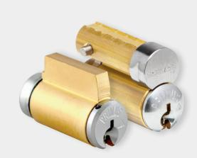
Everest 29<sup>™</sup> SL cylinders are capable of accepting the same Schlage A2 7-pin key system used in SFIC cylinders. Schlage<sup>®</sup> can fit seven pins into a full size Conventional or interchangeable core (FSIC) cylinder by utilizing a locking side bar and patented L-pin design. Seven pins provides significantly more keying combinations than normal 6-pin full-size commercial cylinders, making SL ideal for large campuses.
