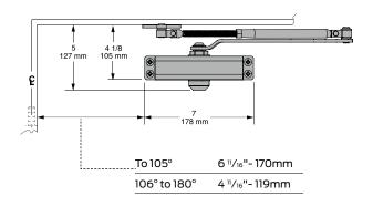
Butt hinges should not exceed 5" (127mm) in width.
