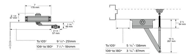
Butt hinges should not exceed 5" (127mm) in width. Auxiliary stop is recommended at hold-open point or where a door cannot swing 180°. Reveal should not exceed 2" (51mm) for regular arm or hold-open arm.
