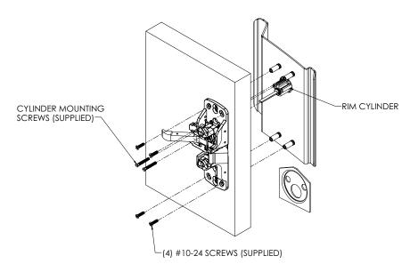
**Note:** When using cylinders other than Sargent, use mounting plates supplied with the cylinder.
