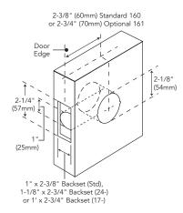
If weather stripping, acoustical materials or silencers are used on the door or frame, care must be taken in the installation so that it will not interfere with the ease in which the latch enters the strike.
