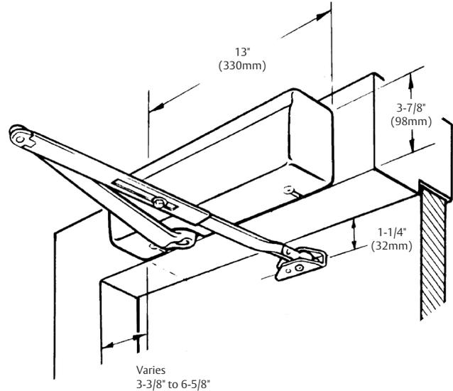
Top Jamb applications - The 351 closer is mounted on the frame face above the door. The foot is mounted on the push side of door. This application is for use on exterior doors opening out to protect the closer from the weather.
