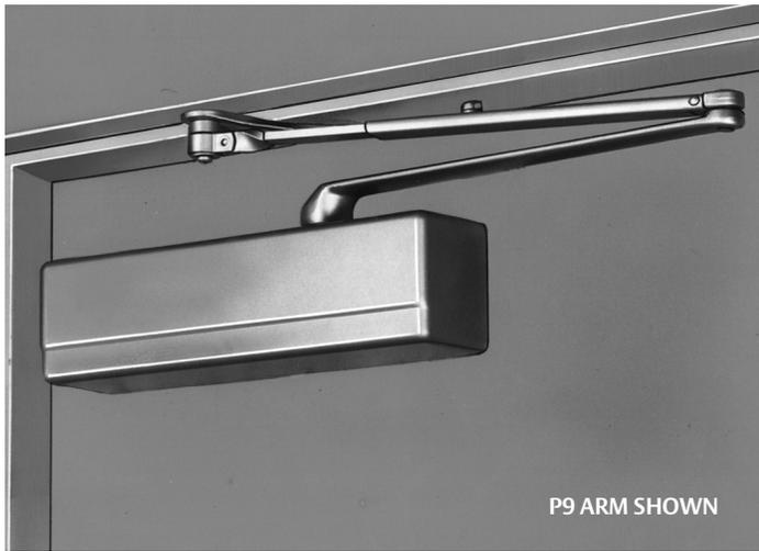
Parallel Arm Applications - The 351 closer is mounted on the push side of the door. As the door opens, the closer swings with the door and gives full headroom in the door opening. Other advantages: the closer arm does not project into the room; the frame can be quite narrow and the door can be swung open much farther than in Top Jamb Applications.
