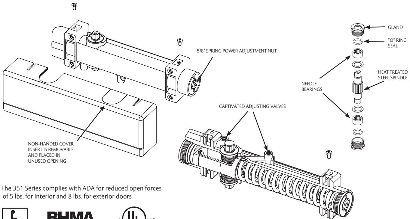
The 351 Series complies with ADA for reduced open forces of 5 lbs. for interior and 8 lbs. for exterior doors
