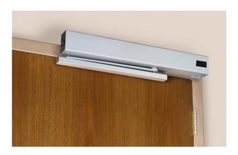
Use a Rixson Smok-Chek® VI style door closer combined with a manifold and solenoid to provide a hold-open feature. When the door is opened manually beyond an adjustable hold-open point and released, the solenoid is energized and the door will remain open.
