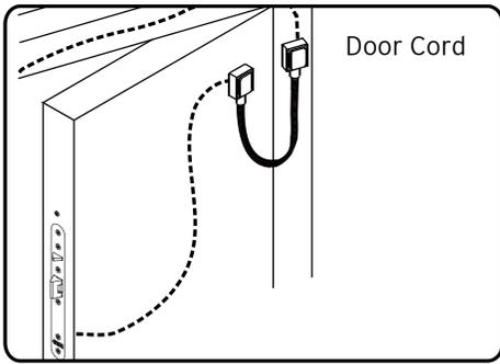
The door cord protects the wiring from damage at the door hinge.
