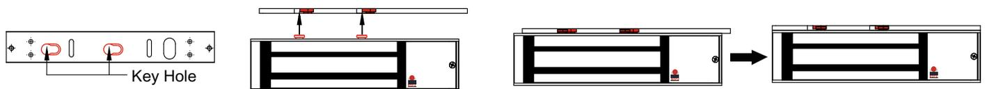
1. Align the two slotted holes and attach the magnet to the mounting plate.
