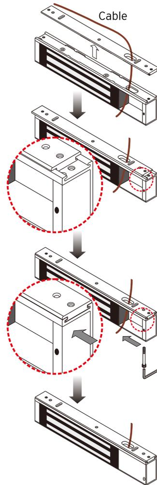
Pass the power cable through the mounting plate and the hole of the maglock.
