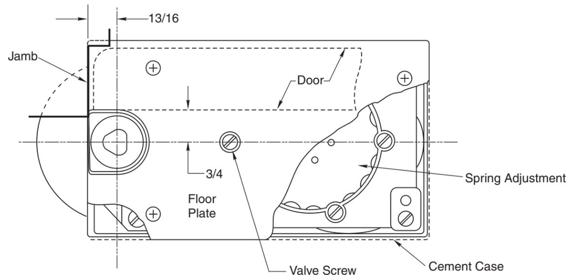
Closing speed can be adjusted to suit local conditions and requirements. With a screw driver turn the adjustment screw that projects through the floor plate or threshold, either in or out as the case may be until the desired action is attained. Turn this valve screw to the right, clockwise, to decrease
