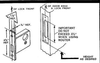
BORE REQUIRED HOLES FOR CYLINDER AND TURN KNOB AS INDICATED IN CHART.
