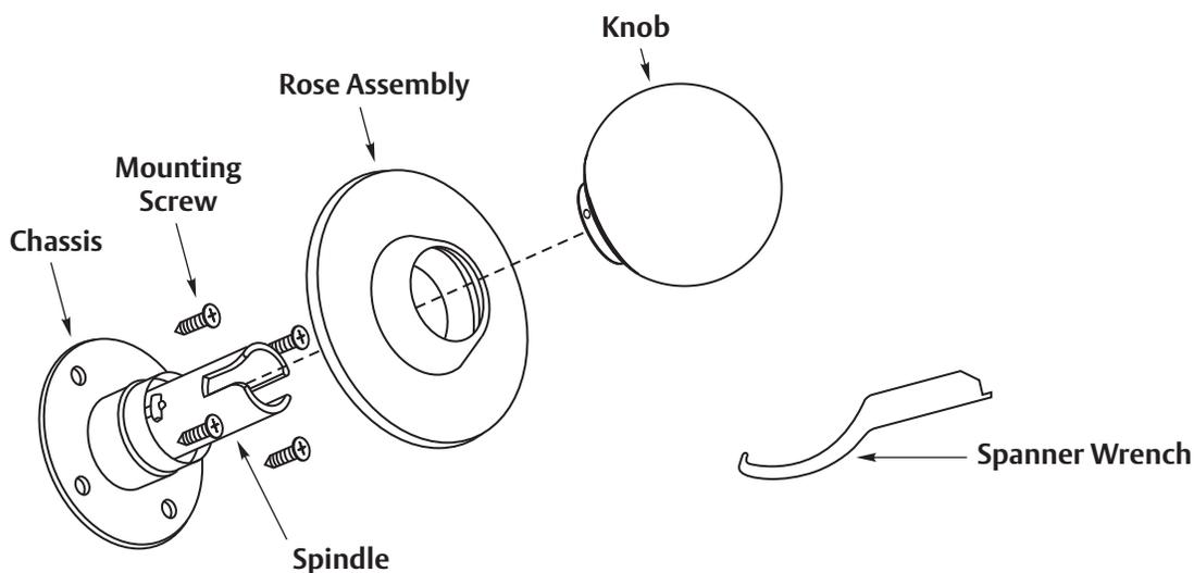
1. Place chassis at proper position on the door (knob retainer facing edge of door) and secure with mounting screws.
