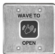
8310-810D Touchless Actuator, Double Gang • Stainless steel • 2 - 24" range • Heavy duty applications
