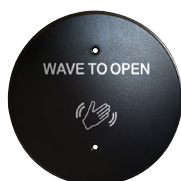
8310-813R Touchless Actuator, Round • Black: ASA, nylon, PC • 4-24" range • Medium duty applications
