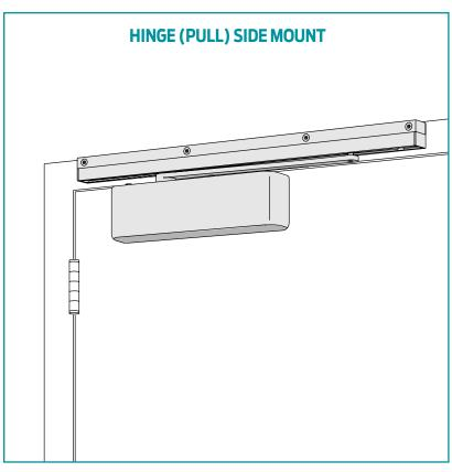
The 4510T SMOOTHEE® Series is a heavy duty, high security track closer with special components to minimize tampering and vandalism. Forged steel single lever arm and heavy gauge metal security cover are designed for correctional, vandal prone, institutional and other high traffic interior applications. The closer has passed 10 million cycles in independent testing. A choice of finishes and cylinder functions meet correctional and vandal resistant requirements.
