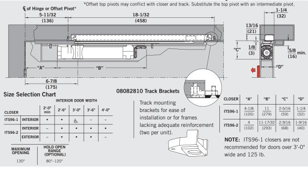
**Note:** These technical drawings are not intended to be used to prepare the door and/or frame. Use installation templates for that purpose.
