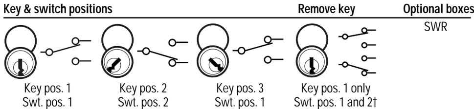
†Installing the limiting plate limits key removal to switch position 1 or 2. The key is always removed in the vertical position (key position 1).
