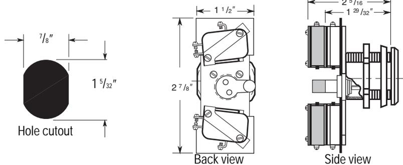
The shaded area shows the additional 1W7R4 switches and cam length.
