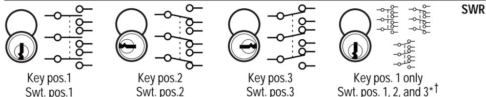
\*Installing the limiting plate limits key removal to switch position 2, or 3. The key is always removed in the vertical position (key position 1).
