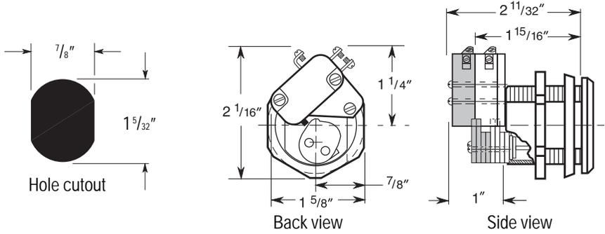
The shaded area shows the additional 1W7J2 switch and cam length.
