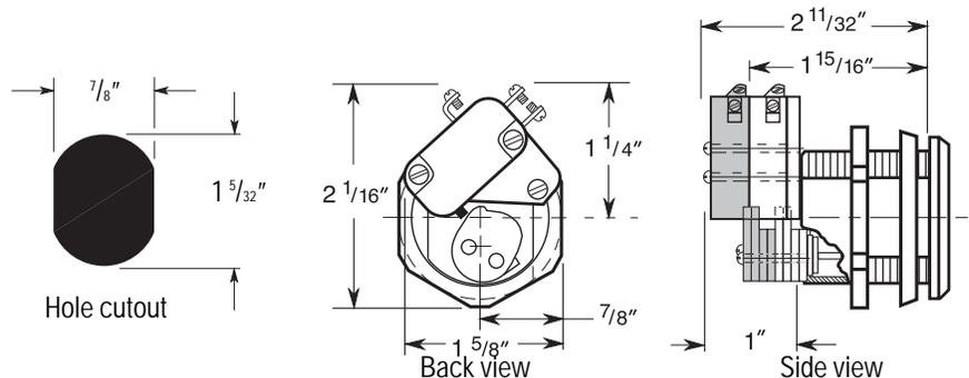
The shaded area shows the additional 1W7J1 switch and cam length.
