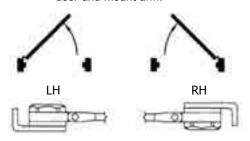
Adjust by loosening hold-open nut, then open door to desired position and tighten hold-open nut securely.
