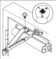
Orient main arm so that the "H", located on the main arm, lines up with the flat on the spindle. Press arm down on spindle and secure with spindle bolt.
