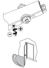
Adjust backcheck accordingly to prevent excessive opening speed.
