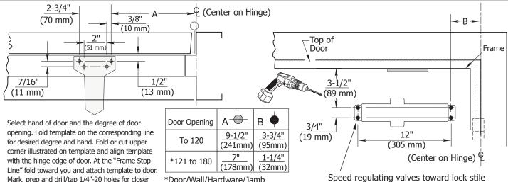
Line" fold toward you and attach template to door. Mark, prep and drill/tap 1/4"-20 holes for closer body and parallel arm bracket mounting screws.
