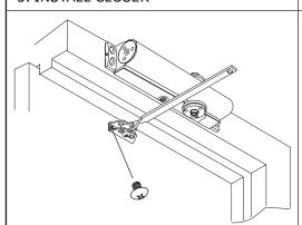
Remove template and use mounting screws to install the closer body to the top jamb and the connecting rod shoe to the door. Closer body should be oriented so that the speed regulating valves are toward the hinge stile of door.
