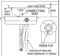
Slide connecting rod into forearm of main arm. Rotate main arm until connecting rod is at a 90° angle to frame. While holding arm in this position, tighten down forearm screw.
