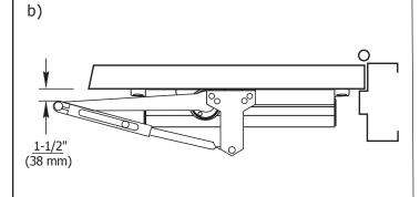
Rotate main arm until the pivot point is 1-1/2" from door surface.
