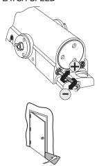
Adjust latch speed so door completely closes and latches.
