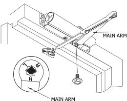
Orient main arm so that the "H", located on the main arm, lines up with the flat on the spindle. Press arm down on spindle and secure with spindle bolt.
