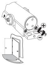
Note: Adjust closing time speed to between 3 and 7 seconds from  $90^{\circ}$  to  $0^{\circ}$ . Greater closing times may be required for elderly or handicapped.
