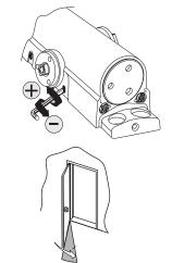
Adjust delay action accordingly to obtain desired delay time.
