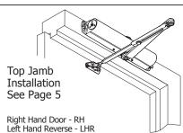
• These door closers should **NOT** be installed on the exposed side (weather side) of exterior doors.
