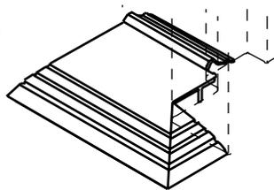
Thresholds are typically installed with the door located above the flat portion of the threshold leaving one bevel edge outside of the doorframe. If simply cut-off it leaves rough cut-away ends exposed on the portion extending outside of the frame and an open area underneath where dirt and debris may accumulate.
