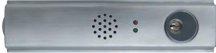
**SIF-EA Exit Alarm** - Slide-In Filler Kit provides 100 plus decibel directional piezo alarm with remote signal relay, remote bypass relay, and LED display. Optional Cylinder Dogging for non-fire rated devices. 9 volt DC and 12/24 volt AC/DC operation. Options include Key Stop feature that allows key to be removed only if unit is armed and factory installed cylinder housing for 7-pin IC cylinders.. Requires mortise cylinder with standard Yale cam (sold separate)
