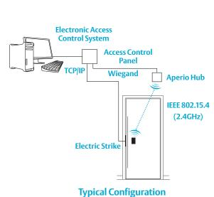
Local wireless communication eliminates the cost and inconvenience of wiring in and around the door, without the hassle of complex site surveys.
