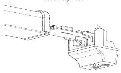
When removing and installing the DSB bar end mount assembly with the PC board from/to the end of the bar, ensure that the lever of the limit switch (under the PC board) does not become dislodged. If the lever is dislodged or comes off, simply reinstall the lever onto the two raised retaining pins of the switch.
