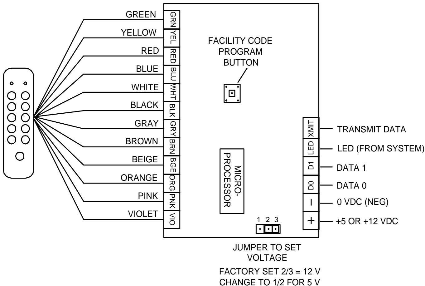
There are 12 color coded wires in the keypad cable. Refer to Figure 1 and connect each wire to the indicated terminal on the CPU Board. No other connections may be made to these terminals (except if two keypads are used with one CPU board).
