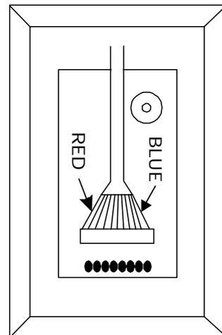
Figure 1 shows the DK-16W CPU Board. You will make connections to the 18 terminals as shown in the drawing and either leave the jumper block in the factory set position (connects pins 2 and 3) if you plan to power the DK-16W with 12 VDC or move the jumper to connect pins 1 and 2 if you will be using 5 VDC. Note that **operation at 12 volts** with the jumper block in the 5 volt position **can damage the unit**.
