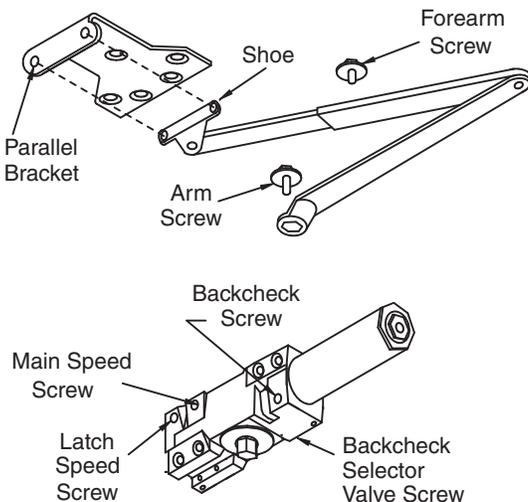
1. Before installation, (parallel arm), turn Back Check selector valve (found on the opposite side of closer) ALL THE WAY IN (CLOCKWISE).
