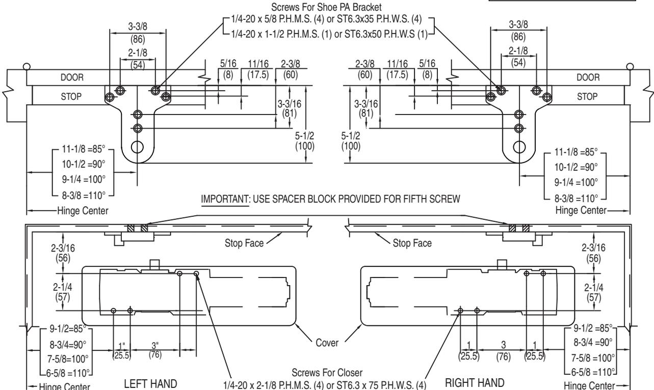
**BEFORE INSTALLING MOUNTED STOP FACE (PARALLEL ARM) TURN BACKCHECK SELECTOR VALVE (FOUND ON OPPOSITE SIDE OF CLOSER FROM REGULATING SCREW SIDE) ALL THE WAY IN (CLOCKWISE)!**
