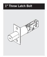
**26170** — 1-1/8" × 2-1/4" front, 1" diameter, 1" throw dead bolt with 2-3/8"-2-3/4" adjustable backset. Square corner. Standard for DB600 Series Dead Bolts.
