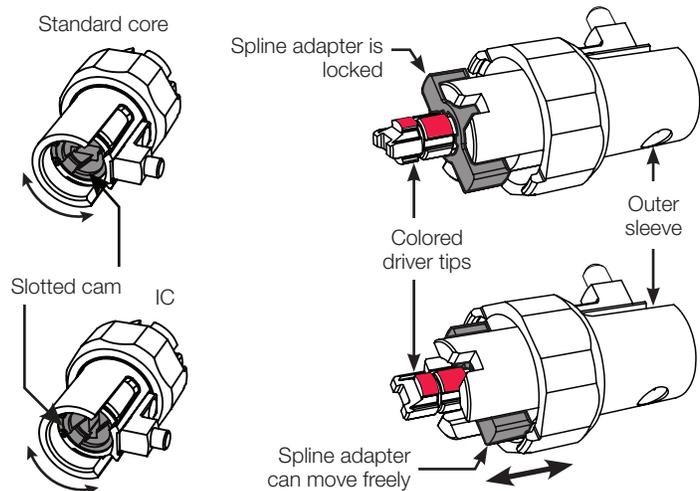
Figure 7 Driver Tip Alignment
