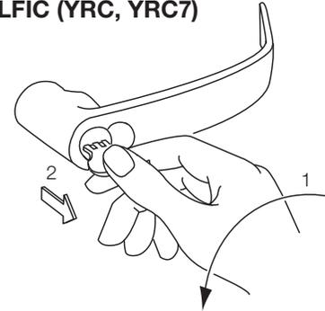
Figure 16 Core Removal
