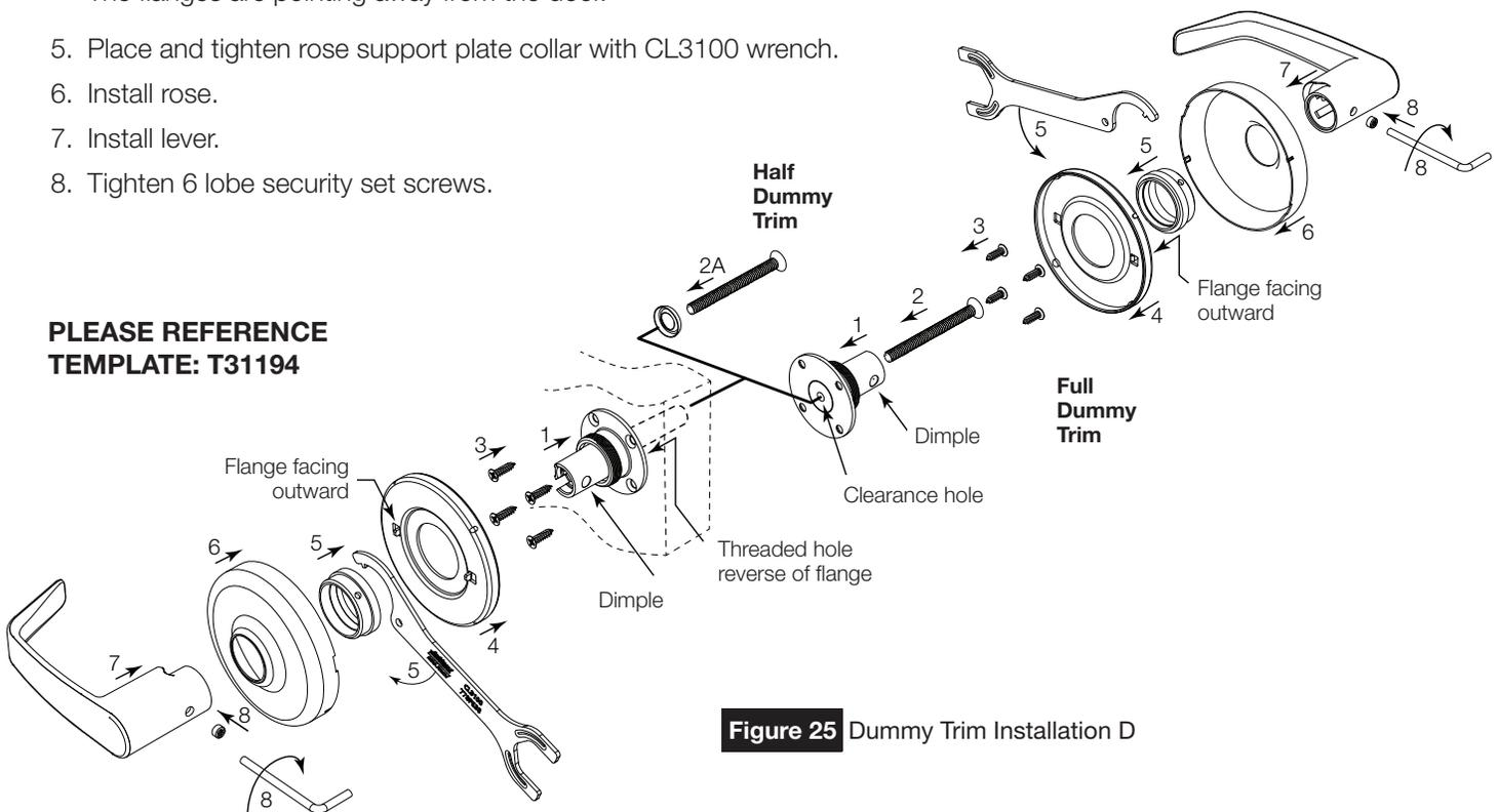
**Figure 25** Dummy Trim Installation D
