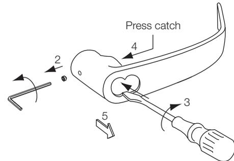
Figure 17 Core Lever Removal
