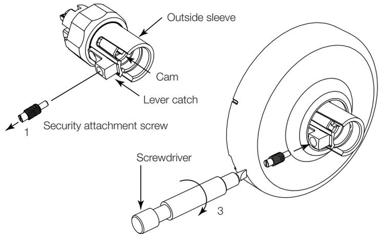
**Figure 21** Security Attachment Screw
