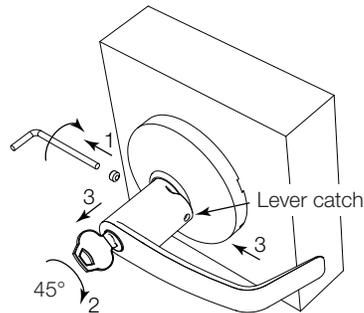
Figure 15 Cylinder Removal
