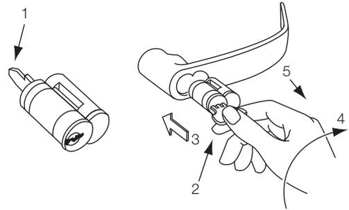
**Figure 19** Core Lever Installation
