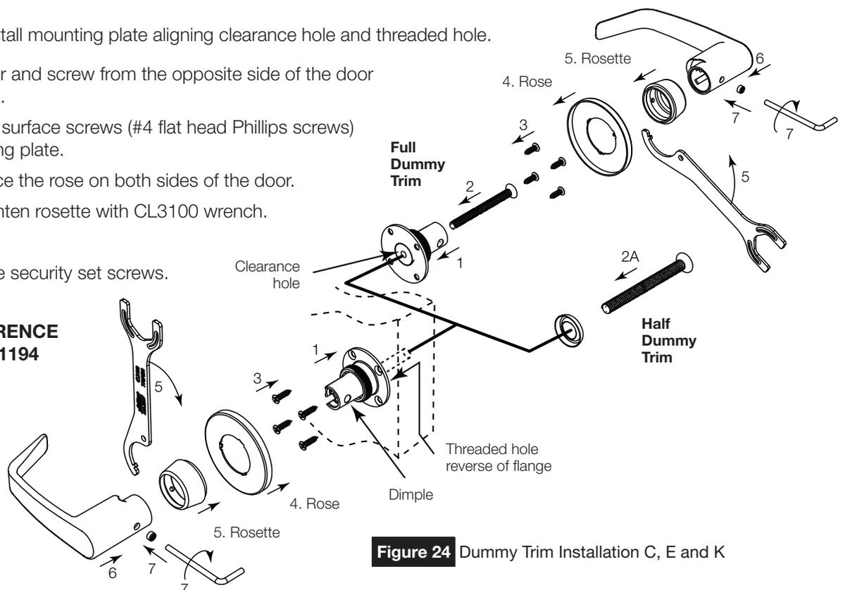
Figure 24 Dummy Trim Installation C, E and K
