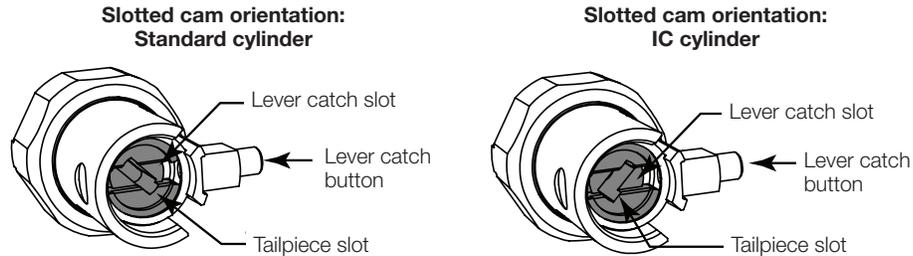
Figure 9 Cam Orientation
