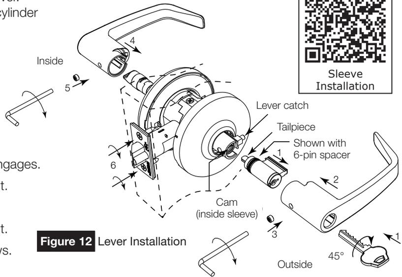
Figure 12 Lever Installation
