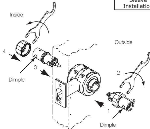
Figure 8 Sleeve Installation
