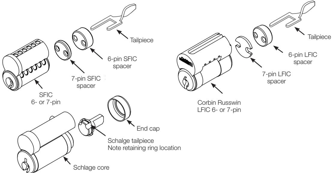
**Figure 20** Tailpiece Installation
