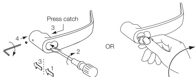
Figure 18 Core Lever Installation
