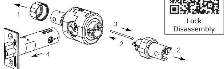
Figure 5 Lock Disassembly
