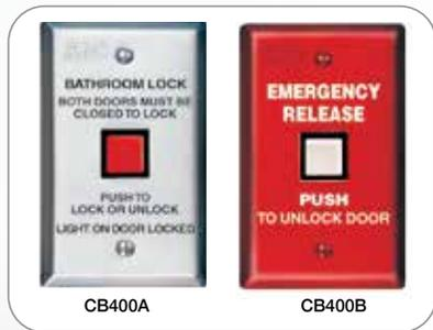
For a common single bathroom shared by two patient rooms or dormitory rooms, the CB400A controls provides privacy and ensures that both doors are locked only when the bathroom is occupied and unlocked when the bathroom is not occupied. The CB400B controls provide emergency access by facility staff. Both doors unlock when signalled by the fire life safety system.
