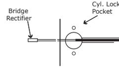
**STEP 5:** Connect the Bridge Rectifier to the plug exiting the cylindrical chassis.
