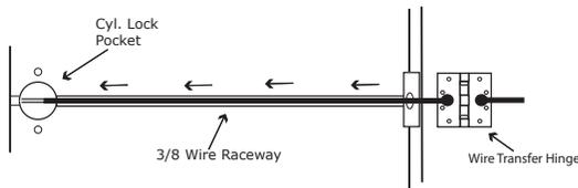
**STEP 3:** Screw the ETH hinge to the door. At this time **DO NOT** connect the hinge wires on the jamb side to the wires coming from the power supply.
