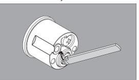
With key removed, insert cylinder into rings (See Step 1) and guide driver bar into slot in latch.
