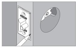
3c Install latch with provided screws.
