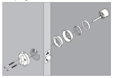
Screw mounting screws from thumbturn through the inside cylinder and tighten evenly.
