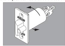
Insert latch into hole. Line up and trace around faceplate.
