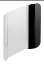
Designed for exterior doors that require extra security or resistance to vandalism, anti-vandal trim (AVT) plates have an extended lip on the active side of the door to provide extra protection for the latchbolt. A matte plastic coated grip provides a comfortable pull over wide temperature ranges. Fully through-bolted with no exposed exterior fasteners for a cleaner look and increased security.
